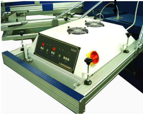
Empty station with flash cure unit
