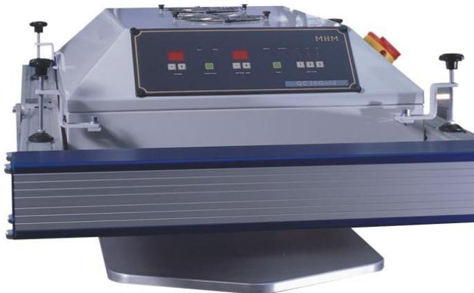
Flash cure units may be installed into either an empty station or a print station. The flash cure unit must be powered by a separate supply, which should comply with the electrical data supplied by the manufacturer (*see data sheet for flash cure units*). To control the unit the dryer must be connected with the dryer connector of the station.
