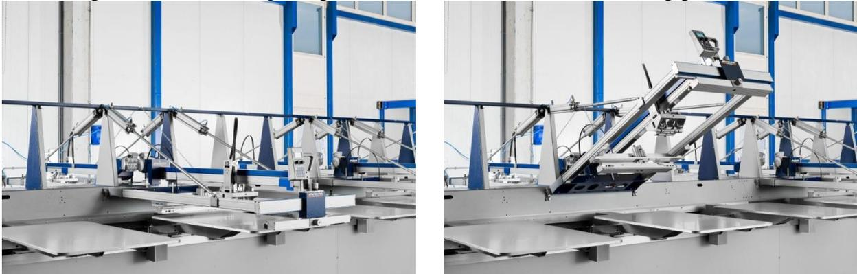
Before lifting a station the squeegee carriage has to be moved manually backwards, until it touches the back Y-axis. With lifted stations the machine must not be depressurized. Don't disconnect the pneumatic line, switching off the machine is no problem. Before reactivating a station (after lowering it) the position of the rear squeegee stroke length adjustment must be checked to avoid a collision between squeegee carriage and Y-axis.
