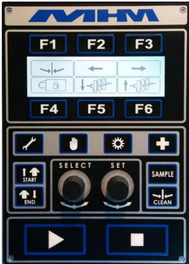
In addition to keys with a fixed function six function keys with various functions are available. The specific action of each function key will be displayed depending on actual function mode. When a function is not possible, the respective symbol will be displayed crossed out. For further adjustment two push- and turning- knobs are available.
