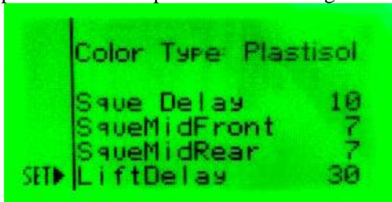
Turning the left knob changes the selected parameter. To choose parameter press the left knob, turning the right knob will change the value. Press the right knob to save the changes. Press the left knob to return to initial value. Exit submenu with button "ADJUST".
