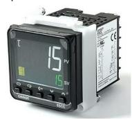
The upper white value displays the actual temperature, the lower green value the adjusted temperature. Use the buttons UP or DOWN to change the adjusted temperature.
